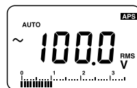
Measuring 100 V using the 300 V range
