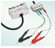
FOUR-TERMINAL PROBE L2000 Cable length 1 m (3.28 ft), DC to 8 MHz, impedance characteristics of 50 Ω, 4-terminal pair configuration, measurable conductor diameter: φ0.3 (0.01 in) to 5 mm (0.20 in)
