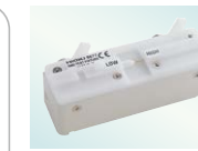
SMD TEST FIXTURE 9677 Direct connection type, For measuring SMDs with electrodes on the side; DC to 120 MHz, test sample dimensions: 3.5 mm ±0.5 mm (0.14 in ±0.02 in)
