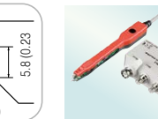
PINCHER PROBE L2001 Cable length 73 cm (2.40 ft), DC to 8 MHz, impedance characteristics of 50 Ω, 4-terminal pair configuration, tip electrode spacing: 0.3 (0.01 in) to 6 mm (0.24 in)
