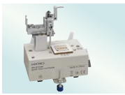
SMD TEST FIXTURE IM9100 Direct connection type, SMDs with electrodes on the bottom, DC to 8 MHz, Measurable sample sizes: 01005 to 0402 (EIA)
