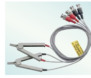
4-TERMINAL PROBE 9140-10 Cable length 1 m (3.28 ft), DC to 200 kHz, impedance characteristics of 50 Ω, 4-terminal pair configuration, measurable conductor diameter: φ0.3 (0.01 in) to 5 mm (0.20 in)
