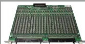
SCANNER BOARD E4201 Semiconductor scanner board with guarding; 128 channels per board *Cannot be combined with other scanner/relay boards.
