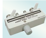
TEST FIXTURE 9262 Direct connection type, DC to 8 MHz, measurable conductor diameter: φ0.3 (0.01 in) to 2 mm (0.08 in)
