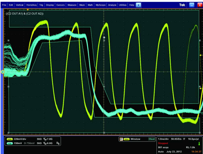
DDR memory. Visual Trigger used to isolate a rare occurrence of a write burst on a specific bit pattern in DDR3. The trigger event is a Write DQ burst of 11000000, when the DQ launch starts from a non-tri-state voltage value. DDR memory bus events involve clocks, strobes and data channels as well as multiple amplitudes and bursts of data.
